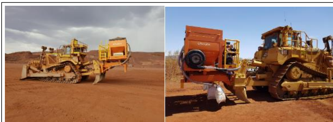
Plate 6. Ellworx machine attached to dozer. Photo credits: Nick Ellwood (Ellworx)
