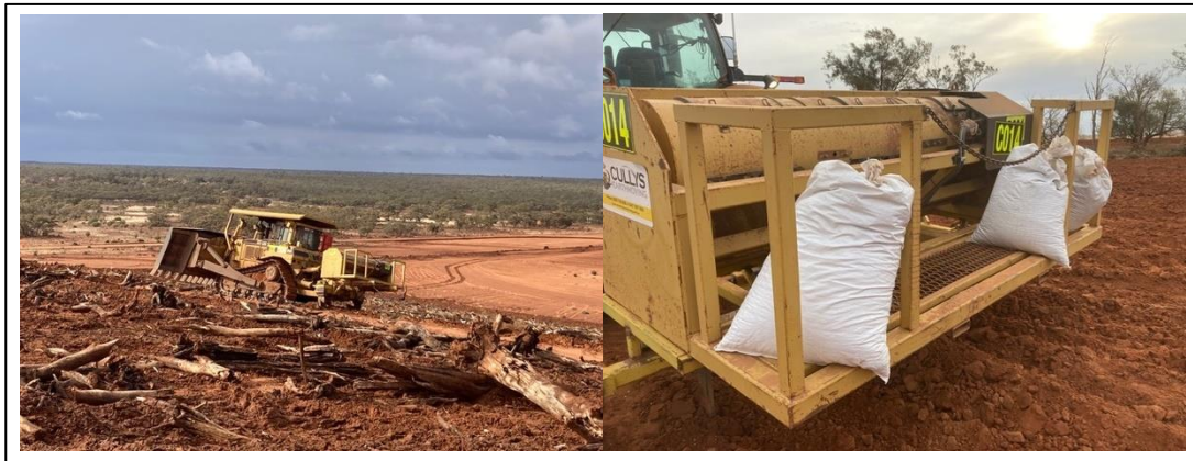
Plate 5. Modified Gessner Drum seeder on bulldozer (Photo credits: T. Zwiersen)
