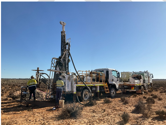
Figure 1 Air core drilling at hole RZCP3289
