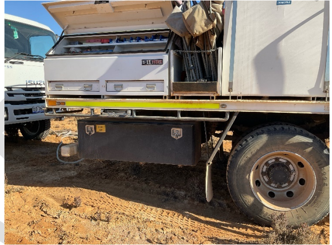
Figure 3 Spill kit in a cabinet beneath the tray of the support truck
